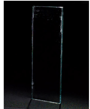
The haze reading for Clarvista® glass in a clear glass substrate was less than 1% after Cleveland Condensation testing.
