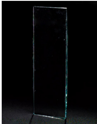
After testing in the Cleveland Condensation chamber, uncoated clear glass had a hazing reading of less than 1%.
