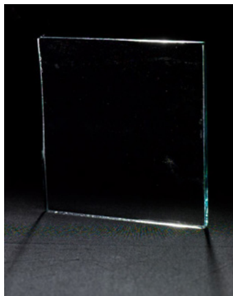
After salt fog exposure, uncoated clear glass had a haze reading of 1%.
