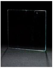
After salt fog testing, *Clarvista* glass in a clear glass substrate had a haze reading of 1 percent.
