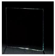
The haze reading for *Clarvista* glass in a clear glass substrate was less than 1 percent after pH/jungle box testing with the ammonia-based glass cleaner.
