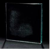
On the leading competitive coated clear glass, pH/jungle box testing with baking soda produced a haze reading of 22 percent.
