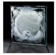
Taber/jungle box testing of uncoated clear glass produced a haze measurement of 83 percent.
