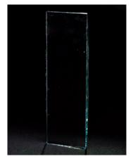
After testing in the Cleveland Condensation chamber, uncoated clear glass had a hazing reading of less than 1 percent.
