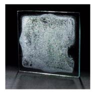
pH/jungle box testing with calcium-lime rust remover produced a haze reading of 58 percent on uncoated clear glass.
