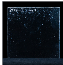
A leading competitor's post-temperable spray-on coating on Starphire Ultra-Clear® glass substrate • Moderate haze
