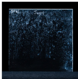
Uncoated glass on Starphire Ultra-Clear® glass substrate • Heavy haze
