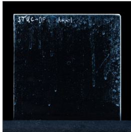
A leading competitor's post-temperable spray-on coating on Starphire Ultra-Clear® glass substrate • Moderate haze
